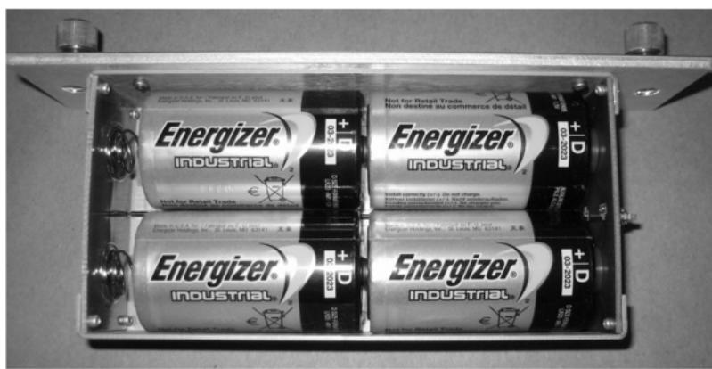
Replace the battery box and tighten thumbscrews.
