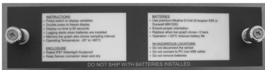
Use new, premium quality Alkaline D-Cell batteries only (Energizer E95 or Duracell/Procell MN1300).
