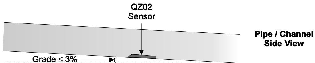
**INSTALLATION – SENSOR LOCATION (Cont.)****1. Flow Profile Distortion**
