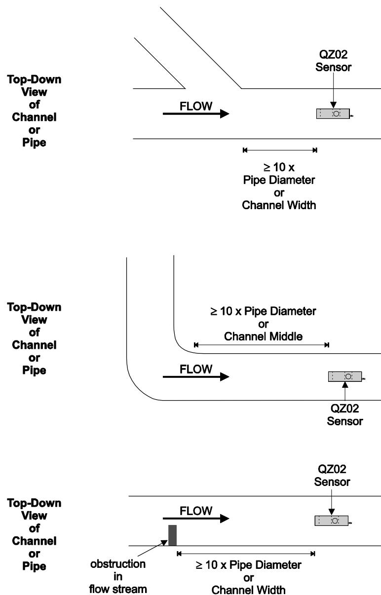
**QZ02L VELOCITY-LEVEL SENSOR MOUNTING**
