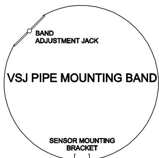
Use optional VSJ stainless steel Pipe Mounting Bands for easy Sensor installation in round pipes.
