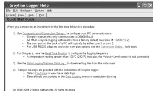
4. Configure Greyline Logger software Communication Settings. Stingray baud rate is fixed at 28800 Baud. Identify the serial port on your laptop or PC. Refer to the Greyline Logger 'Help' file 'Connection Setup' for detailed instructions if you are not sure which COM port or virtual port you are connected to.
