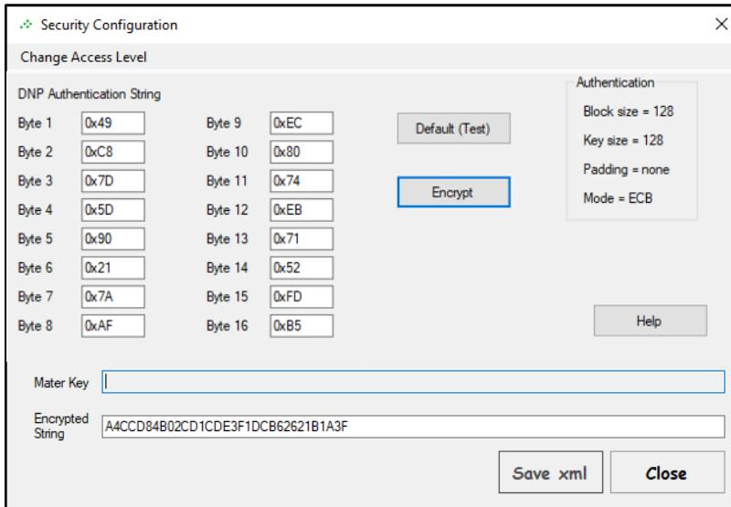
The authentication key for the master is set by populating the text boxes Byte 1 to Byte 16, for initial testing you can default the key, this will populate the Master Key box, to make it easier to copy and paste to a master.
