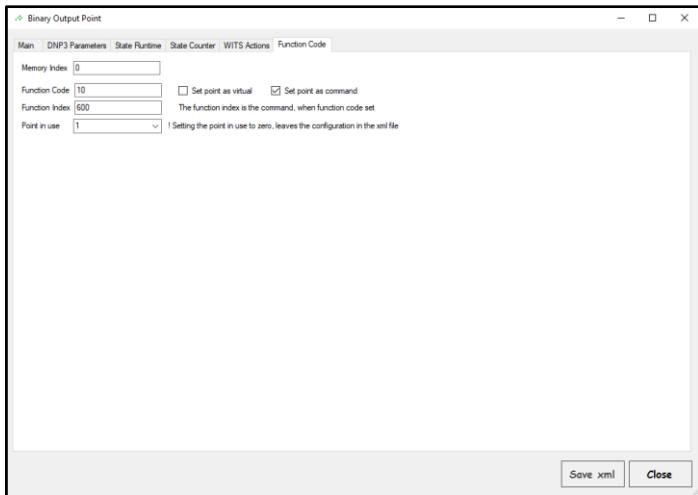
The functionality of this tab is similar to the binary input. However, the difference is that the function code is set to 10, and the function index is 600, which comes from the excel spreadsheet of Ultimate Controller remote commands (this is Run on enabled).
