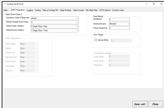
The functionality for the group boxes Static/Event/Class 0 and DNP3 Flags have been explained previously in the manual. For further information on their functionality please refer to the [Binary Inputs Open data points](#) section of this manual.
