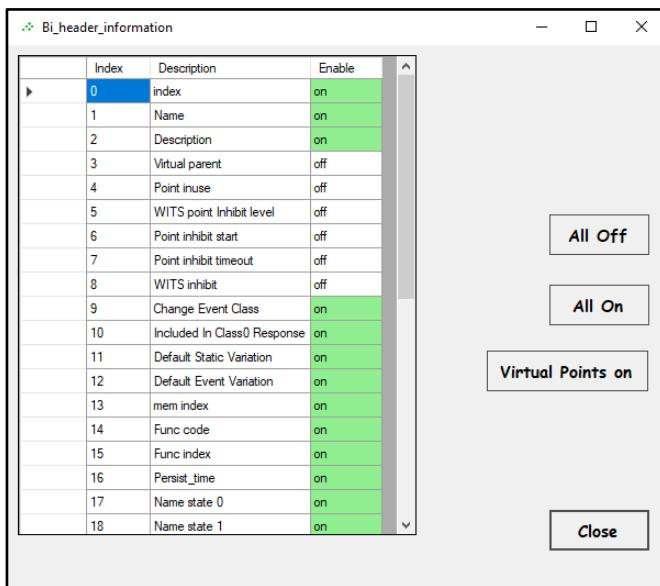
Selecting this option will allow the user to adjust which variables are shown in the points in the Binary Input table.
