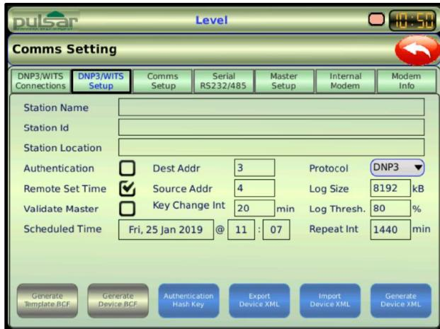
To export the xml file to the SD card, press the **Export DNP3 Device XML** button to begin the export process to the SD card. The file will be saved on the SD card as an rtu.xml file on to the SD card, which can be used to set up another Ultimate or read and changed using the Pulsar DNP3 software.
