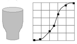
You should enter 2 level/volume breakpoints at the minimum and maximum levels, and several for each place where the vessel has got an arc. You can enter any number of pairs between 2 and 32.
