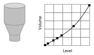
You should enter a level/volume breakpoint for each place where the vessel changes direction, and numerous where the section is slightly curved (mostly linear but has got a small arc). You can enter any number of pairs between 2 and 32.
