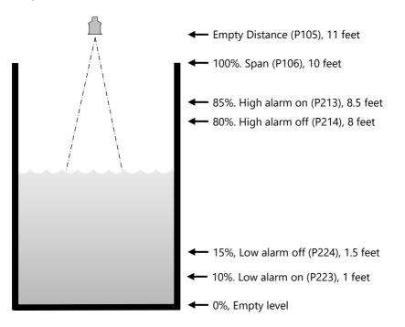
In this example, when the level rises to 8.5 feet, relay 1 will come on until the level drops to 8 feet when it will turn off. If the level drops to 1 feet, then relay 2 will come on until it rises 1.5 feet when it will turn off.
