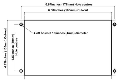
The dimensions of the wall fixing holes are as shown below:
