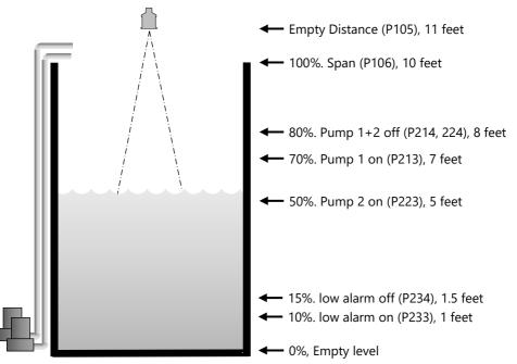
In this example, there are two pumps, which will be set to **alternate duty assist**, so they come on alternately. Pump 1 is to be set to relay 1, pump 2 to relay 2, and the high-level alarm to relay 3.
