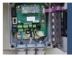
WSI decided to replace the existing IMP 3 with an IMP 6. This proved to cope with the measurement depth much better as the IMP 6 has a measurement range of 6 m and can provide the accurate reservoir level readings the airport was looking for.
