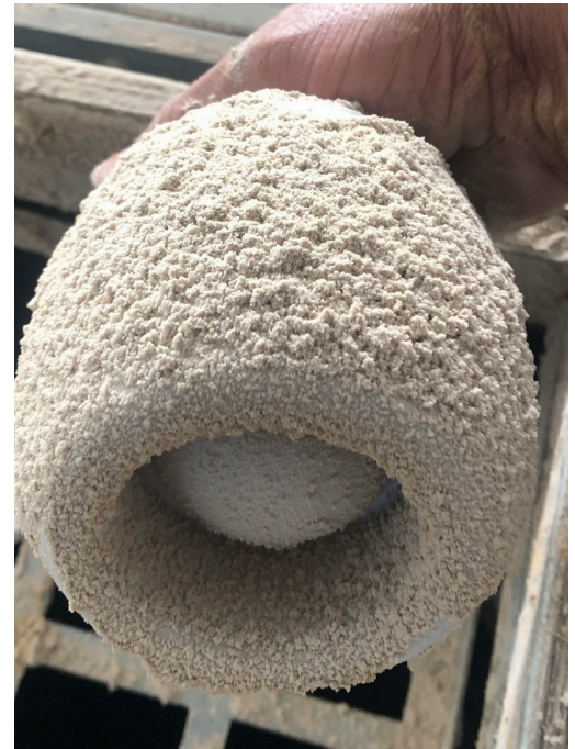
A REFLECT™ sensor covered in debris from the silo, but still able to provide accurate readings.
