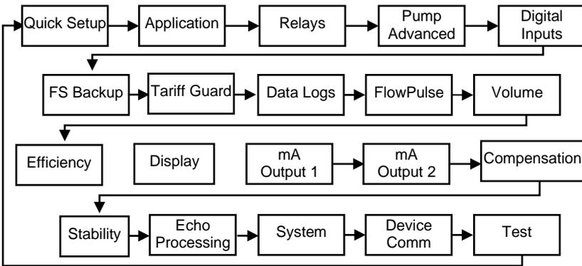
As you press the cursor keys to scroll left and right between these, you can press ENTER at any time, to select the desired menu heading, and take you to the sub-menu.
