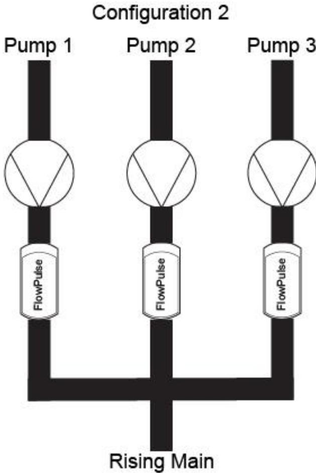
In configuration 2 each of the FlowPulse will be allocated to the pumps they are attached to. Without a FlowPulse allocated to 'All' the summation of flow being measured by all FlowPulse will be used to totalise and output flow.
