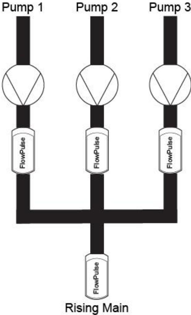
Configuration 3 has a FlowPulse allocated to each pump and a FlowPulse attached to the 'Rising Main' allocated to 'All'. In this situation although there are FlowPulse attached to the pumps, the FlowPulse attached to the 'Rising Main' and allocated to 'All' will be used as the output for flow and totalising.
