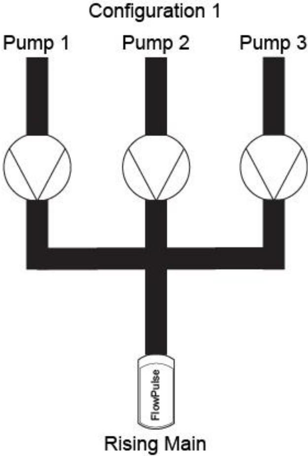
In configuration 1 the FlowPulse attached to the 'Rising Main' should be allocated as an 'All' FlowPulse (P1131, P1151, P1171, P1191). This will ensure that this FlowPulse is the only one used to totalise and output flow.
