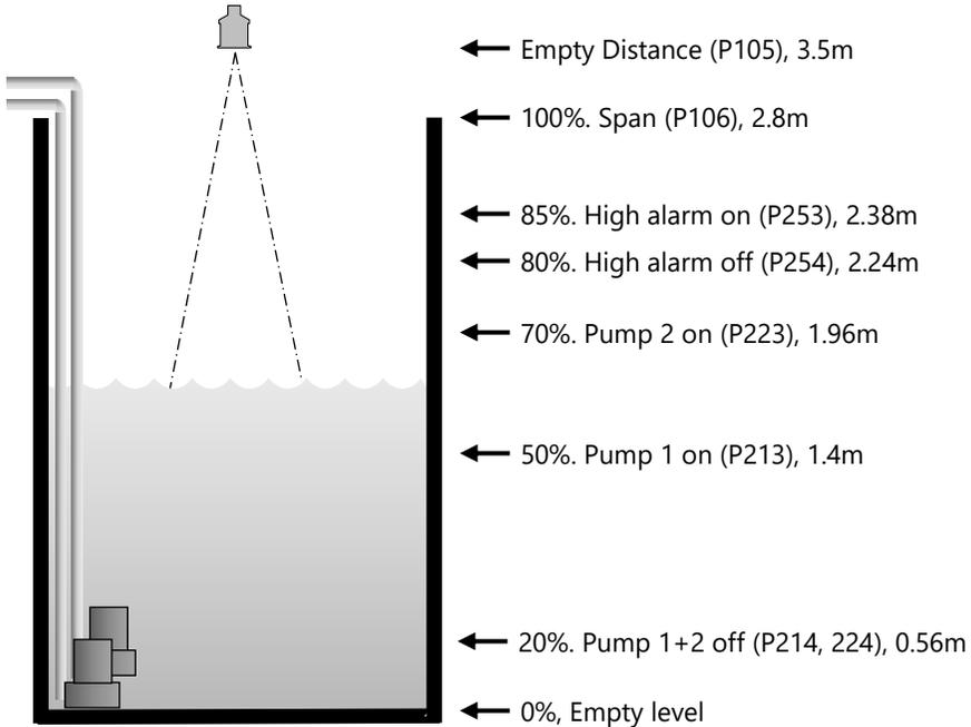
In this example, there are two pumps, which will be set to **alternate duty assist**, so they come on alternately. **Pump 1** is to be set to **Relay 1**, **Pump 2** to **Relay 2**, and the **high-level alarm** to **Relay 5**.
