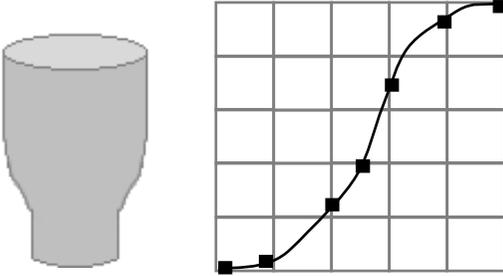
You should enter 2 level/volume breakpoints at the minimum and maximum levels, and several for each place where the vessel has got an arc. You can enter any number of pairs between 2 and 32.
