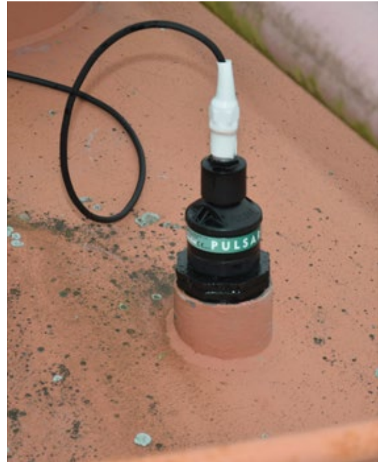
dB6 with front-nose threads for easy connection to an existing outlet on the top of the tank
