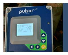
The DFM 6.1 performed perfectly, picking up flow rates of around 7 m/s which was in line with the customers' expectations. The flow meter met the needs of the enduser and was within the budget for the product.
